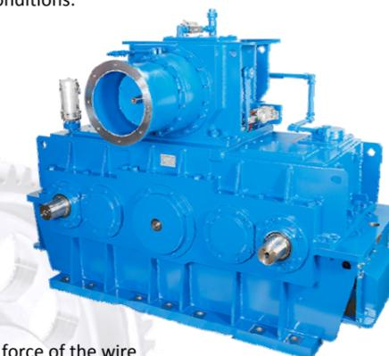
This gearbox is designed for a maximum output torque of 214.000 Nm. In this case two main operation conditions, plus the output shaft bearing coping with the force of the wire drum, are met in one gear unit together with the explosion proof oil lubrication system. The fabricated housing is built for extreme operation temperatures from -56°C to +60°C. These special designed gear unit weighing 9 tons is a guarantee for a long lifetime and reliable function even under extreme conditions.
